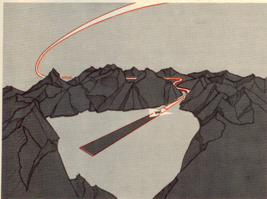
Figure 10. The landing approach path may be determined by the terrain and may bear little or no resemblance to the standard pattern.
